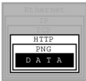
Figure 2. Sockets Covered Protocol Layers
